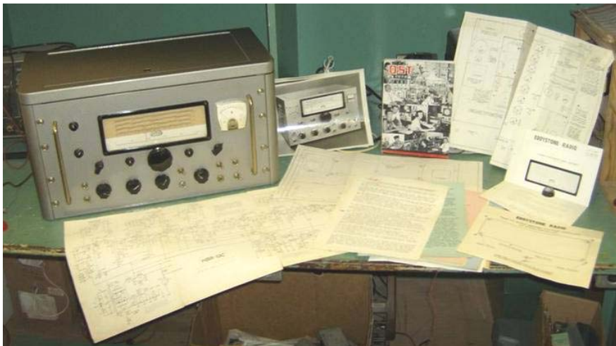
Above: The HBR13C donated to the SPARC museum. Built in 1965/66, it came with an extensive set of documents used in its construction – some laid out in this photograph (though the coil winding tables were not included). Also shown here is the copy of QST (October, 1965) containing the article on this variant of the HBR receiver series (see photo at top of this page)
