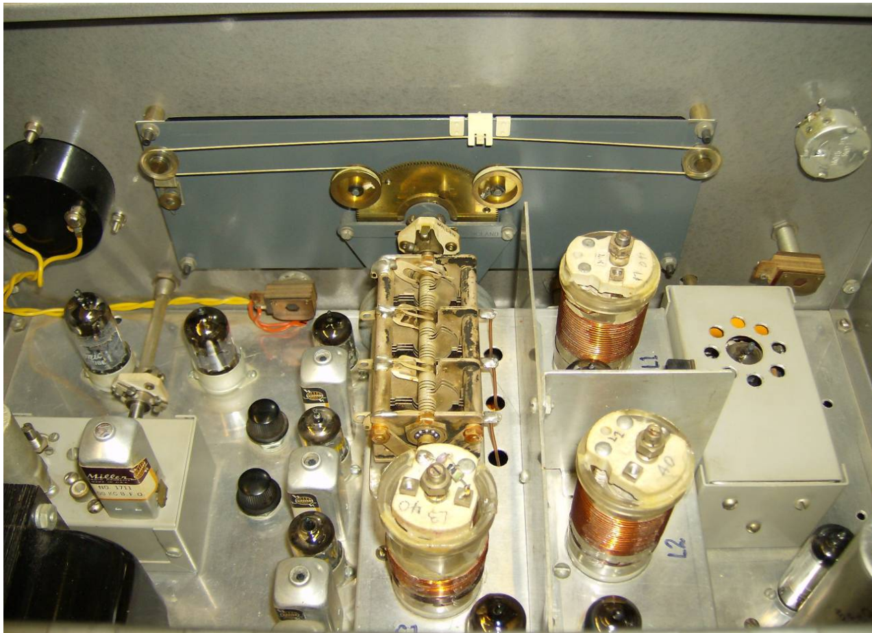
Above: An above-chassis view into the HBR13C – note the 40 metre coil set is fitted here (L1. L2, and L3). The Eddystone '898' can be seen coupled to the tuning gang via a Millen flexible coupling
